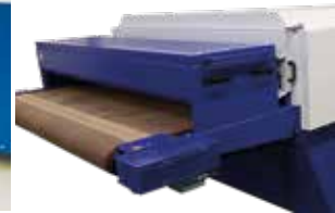
Optional cooling bridge over the outlet
